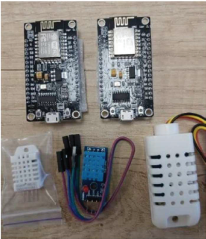
Fig.13. Temperature and humidity sensors DHT11, DHT22, with the ESP8266 microcontrollers.
