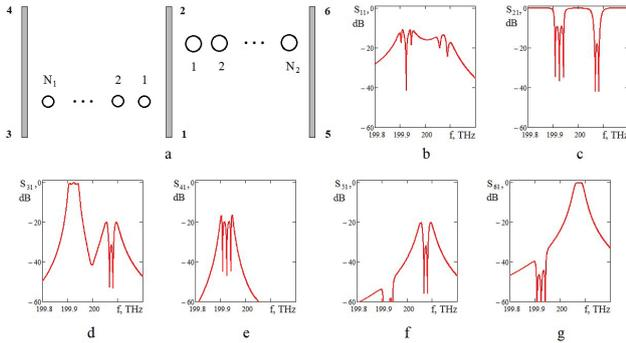
Fig. 4. Diplexer on two different bandpass add/drop filters (a). Scattering characteristics (b - e) of filters (b - g). Coupling coefficients between neighbouring resonators of the second filter: for even mode:  $k_{12}^{2e} = 1,4 \cdot 10^{-4}$ ; for odd mode:  $k_{12}^{2o} = -1,4 \cdot 10^{-4}$ . The remaining parameters of the resonators are as in Fig. 3.
