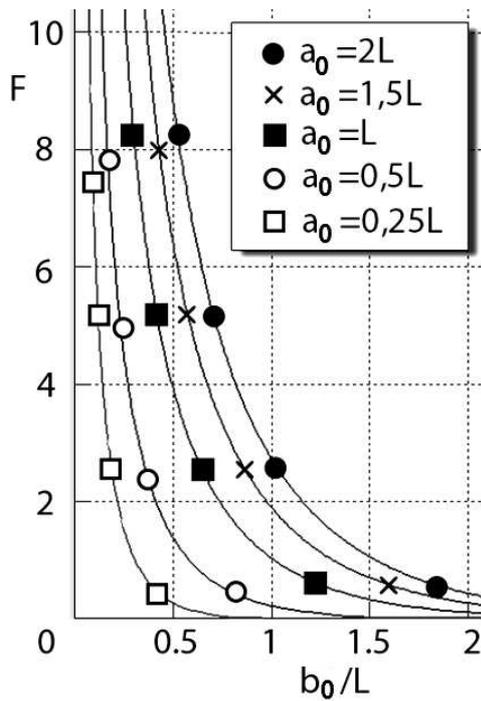
Fig.2. Normalized resonant frequency of the rectangular DR
