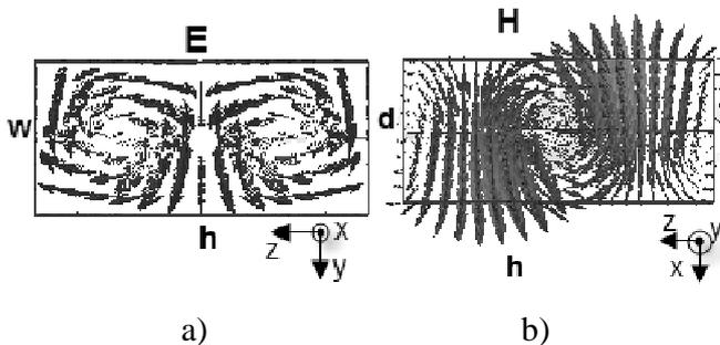
Fig.3. Distribution of electro (a) and magnetic (b) fields of TE<sub>218</sub> at frequency of 5.58 GHz
