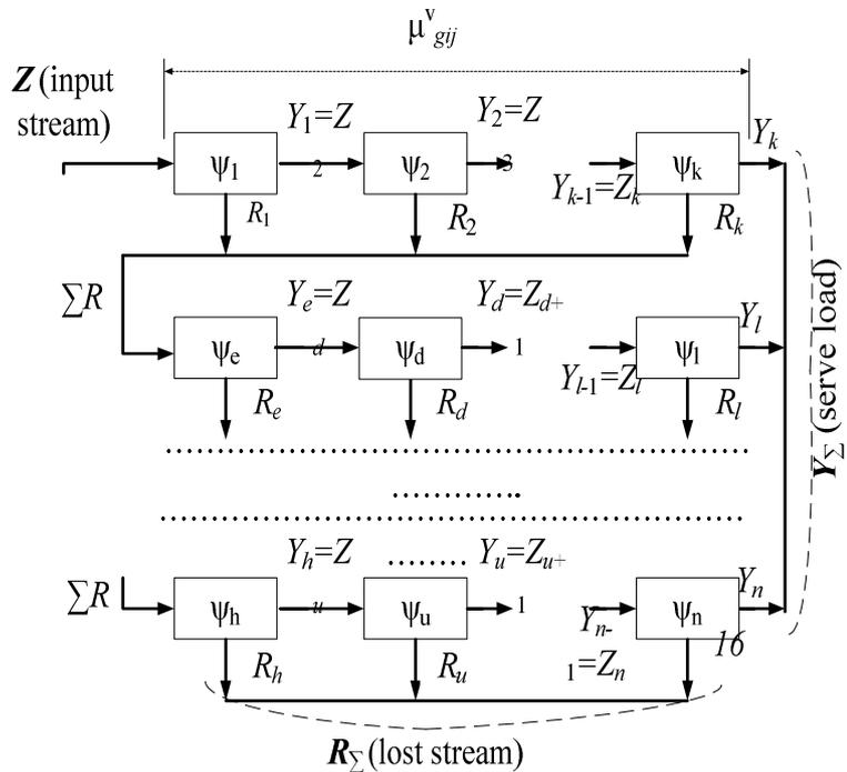
Fig. 3. Model functioning MPLS network in the direction of communication
