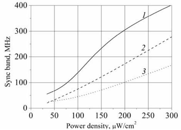
Fig. 8. The width of external synchronization band for single active antenna (1) as well as for linear arrays consisting of two (2) and three (3) mutually synchronized antenna-oscillators versus the power flow density of the external signal.
