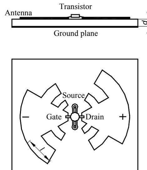
Fig. 1. The structure of active antenna with field-effect transistor.
