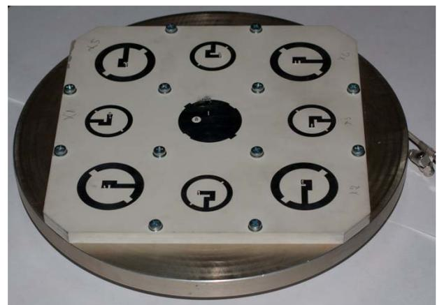
Fig. 6. Manufactured test sample of 10-element dual band circularly polarized switched smart antenna array. The central element for  $L2$  band is hidden.
