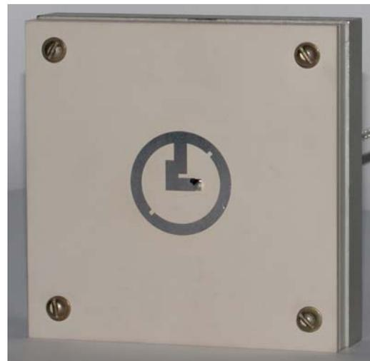
Fig. 2. Photo of manufactured standalone annular ring radiator designed for operation in the  $L1$  band.
