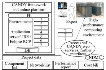
Fig. 7. Design tool integration and access with the following modules: (1) project manager; (2) network editor; (3) component browser; (4) SCS trace router; (5) wireless site finder; (6) workload analyzer; (7) bill reporter; (FE) front-end via XML; (T) loose-coupled and 3rd party tools, like, for instance, NS-2; (DB) component repository.
