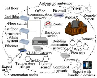
Fig. 6. A combined office communication and building automation network.
