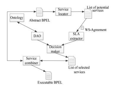
Fig. 1 Architecture of software environment for SLA-aware WSC
