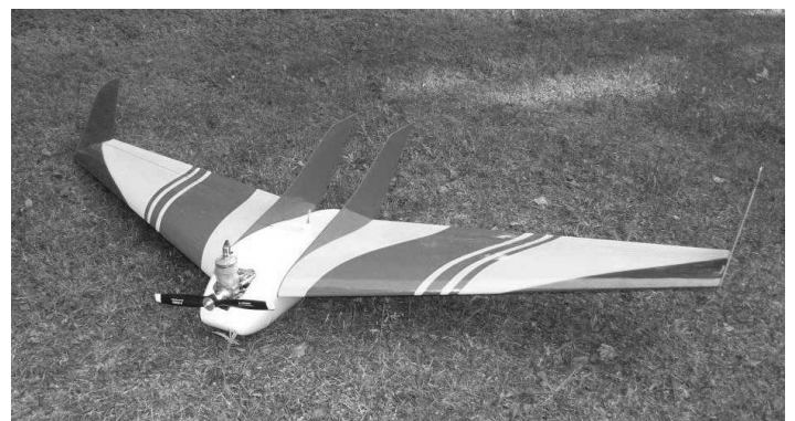
Fig.2. Miniature UAV prototype (developed in National Technical University of Ukraine “KPI”)
