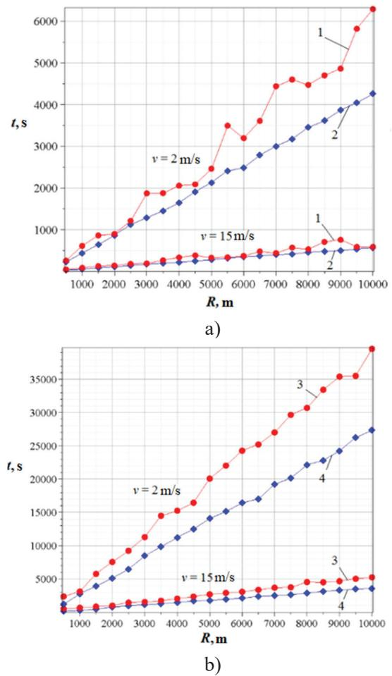
Fig. 11. Dependence of the average time for a MS to reach the limit of the coverage area on its radius at different speeds and movement scenarios: 1 – "march" (a), 2 – "incoherent" (a), 3 – "random wandering in the field" (b), 4 – "random wandering in the city" (b)
