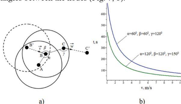
Fig. 7. The model (a) and the calculation results of connectivity duration with one retransmission (b)
