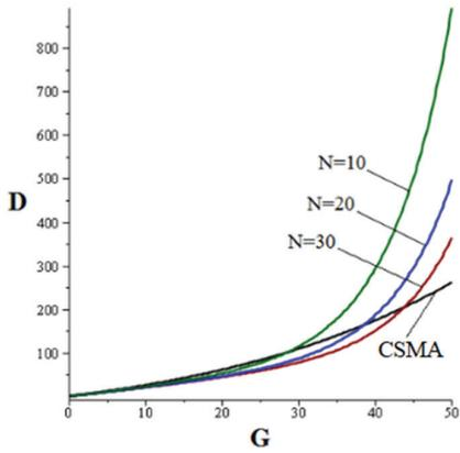
Fig. 4. Graphs illustrating the dependence of the average transmission delay of one MS-MS link (at  $x=1000$  m) and one UAV-UAV (UAV-MS) link (at  $x=5000$  m,  $N=5,10,15$ ) on traffic intensity
