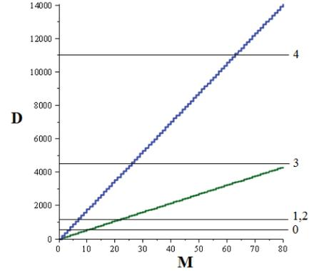
Fig. 5. Graphs illustrating the dependence of average end-to-end packet transmission delay through MS network (1) and through UAV network (2) with indication of QoS levels (ITU-T Y.1541)
