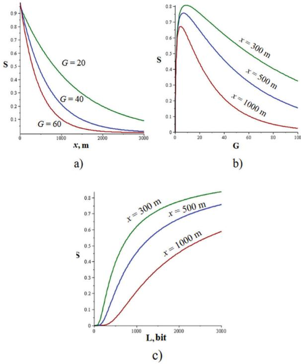
Fig. 2 - Graphs illustrating the dependence of the bandwidth of the MS-MS channel on: a) - the distance between nodes at different values of traffic intensity, b) - the traffic intensity at different values of distance between nodes, c) - the packet length at different values of distance between nodes (at  $G=40$ )
