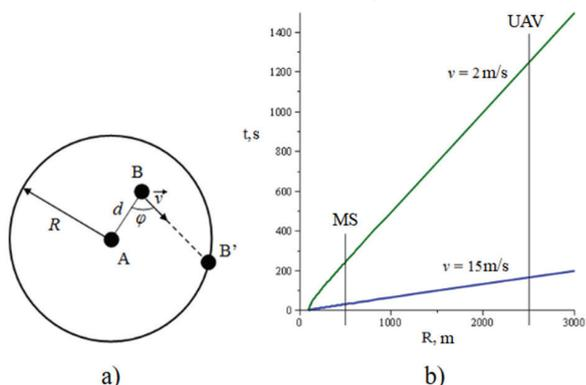
Fig. 6. The model a) and the calculation results of connectivity duration b)
