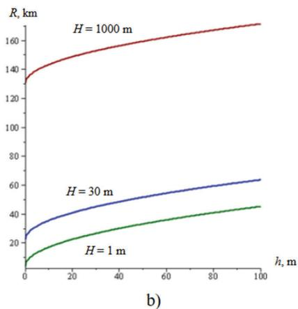
Fig. 1 - Range of direct visibility considering the height of the suspension of antennas with different correction factors: a) -  $K=1$ , b) -  $K=4/3$
