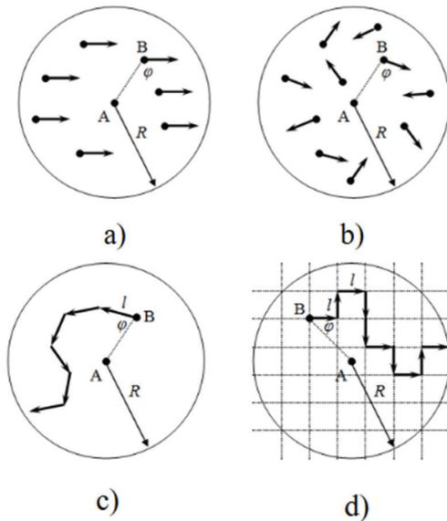
Fig. 10. Movement trajectories of WEN nodes depending on the mobility scenario: a) - "march", b) - "incoherent", c) - "random wandering in the field", d) - "random wandering in the city"
